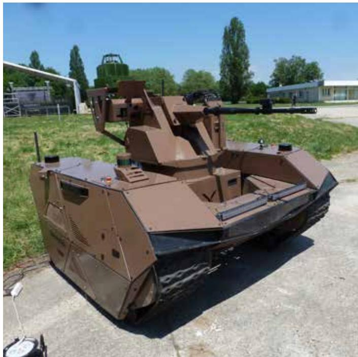
*The OPTIO-X20 armed unmanned ground vehicle developed by Nexter and based on the Milrem Robotics' Themis tracked platform. UGVs will be come an increasingly important asset in the near future.*
