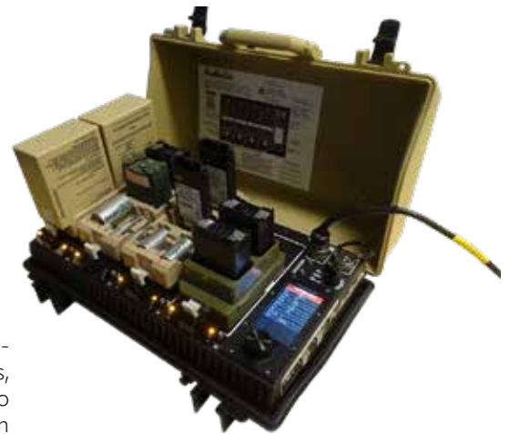
As an example, the BTC-70100 can charge eight BB-2590/U batteries from 0% to full in less than 3 hours, and 16 Conformal BB-2525/U batteries in less than 3.5 hours.
