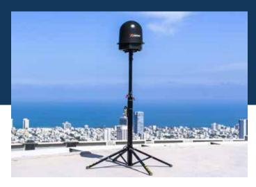
of frequencies; the older models had detection in the 400, 800 and 900 MHz bands, and direction finding and detection in the 2.4 and 5.8 GHz bands, while the new one ensures all functions including identification in all five bands, the lower ones being the most used by do-it-yourself drones. Thanks to new algorithms accuracy and range perfor-
