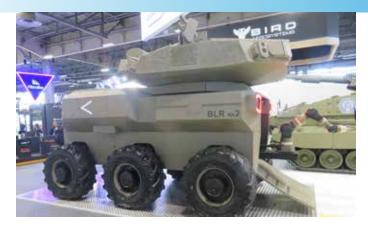
velopment by the Israeli MoD and a number of Israeli companies. The technical demonstrator includes a new robotic platform from BL, a 30 mm autonomous turret developed for the "Eitan" APC, Elbit's "Iron Fist" Active Protection System, fire control and mission management systems, and robotic autonomous kit, in addition to situation awareness systems.
