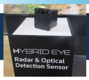
Hybrid-Eye integrates a C-band phased array radar, multiple infra-red warning detectors in different frequency bands, and a laser warning detector into a rugged 16x16x11cm enclosure weighing less than 4kg. Bird's fusion software combines the information from all the sensors to provide a multi-band solution that can detect, alert, confirm and track multiple threats and cue the response in a cluttered environment.
