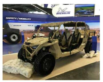
high-strength polymer spokes, that carry the load and absorb impacts helping dampening the ride, increasing comfort and allowing higher crosscountry speed. Airless tyres are more robust, last longer, and do not fear punctures, hence small arms fire, but no specific details were yet provided on specific tests in military environment.
