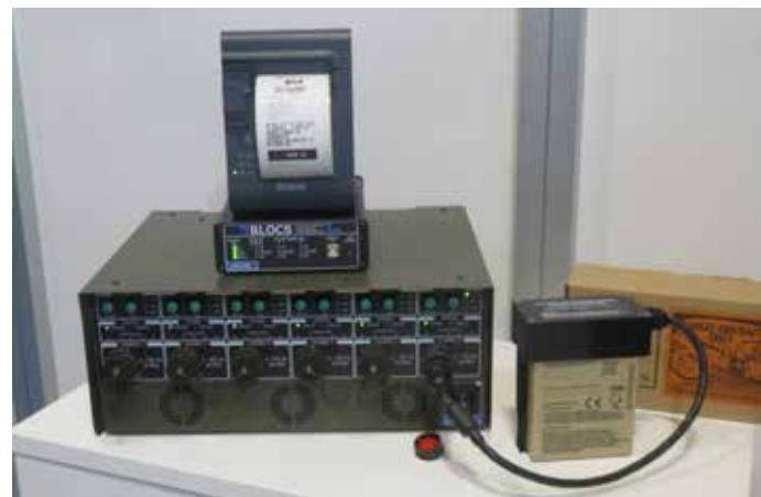
192 batteries can be processed and labelled simultaneously using Lincad's six-channel Armada conditioner.
