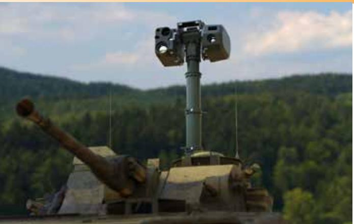
rios. It also includes a proven, easy to use and intuitive visual interface, which presents clear images of objects of interest. Hawkeye MMP can also be connected to a combat management system to hand off and receive targets quickly and effectively, considerably enhancing mission performance. The system uses 'a single head' with rapid removal and replacement of the quick fit pods for mission role changes, which removes the need to hold dedicated vehicles or systems for those specified roles.
