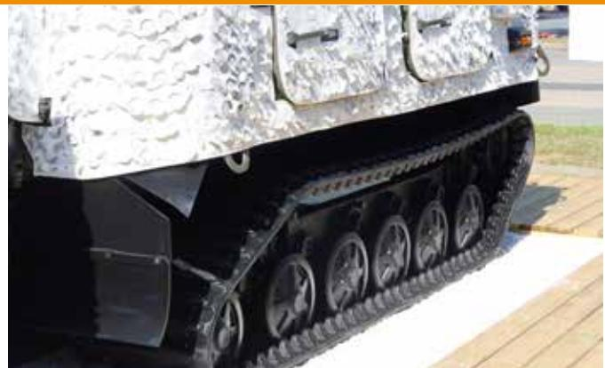
**S**oucy's latest improvements are major step forward in their capability and opens the door to a previously unavailable market segment, such as tracked self-propelled artillery systems and light tanks. The company announced the latest iteration of its rubber tracks, which can be used on tracked platforms weighing up to 55 tonnes. Soucy leveraged its over 50 years experience of rubber track design in the civil segment and com-
