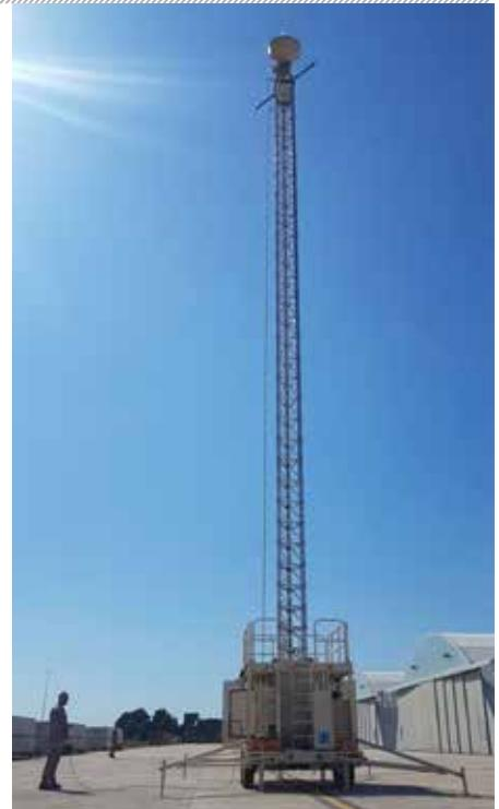
resistant trailer transport frame specially designed to transmit and endure the high loads and moments transferred to the trailer by a tower mast subjected to the forces of wind and weight of gravity. Air transport is supported by US Air Force ATTIA (Air Transportation Test Loading Activity) and by Italian Air Force certification. ■
