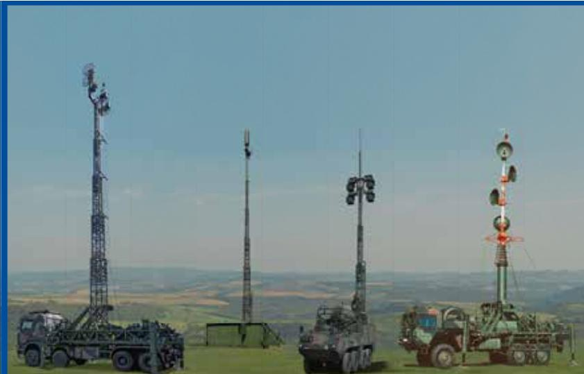
Your reliable partner for daily support, especially for very demanding and important missions. Worldwide the only manufacturer of Mobile Antenna Masts up to a height of 40 m without using any kind of guy wires.
