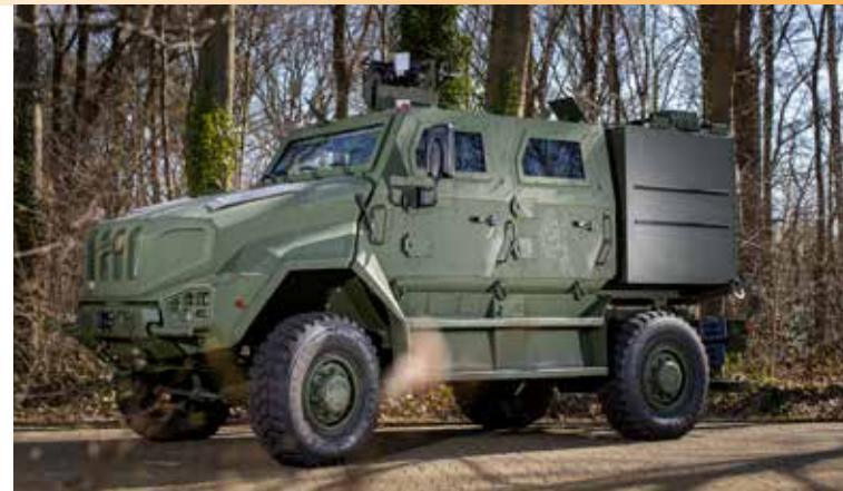
First time Eurosatory presence for the IDV Medium Tactical Vehicle (MTV). Designed to answer a Dutch MoD requirement, IDV signed the contract for what is known in the Netherlands as 12kN in November 2019. In fact, the expected payload of 12,000 N, 1,224 kg, was largely exceeded and is now 2,000 kg, for a kerb weight of 10 tonnes. Powered by a 276 hp engine, it features a ladder chassis with leaf spring suspensions
