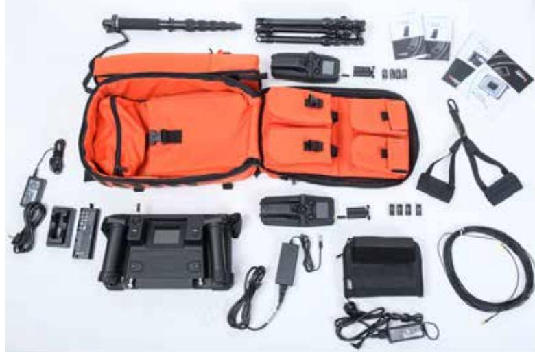
The XaverNet is also part of the rucksack, this being a remote wireless ToughPad that can receive real time visual data and fully control remotely up to four Xaver systems simultaneously at distances up to 200 m, depending on conditions, and also allows a better view on its bigger 7-inch screen. A tripod, a monopod and a spider strap, useful to keep in place the Xavers freeing the operators hands, are also contained in the multi-functional backpack which weighs overall less than 9 kg. ■
