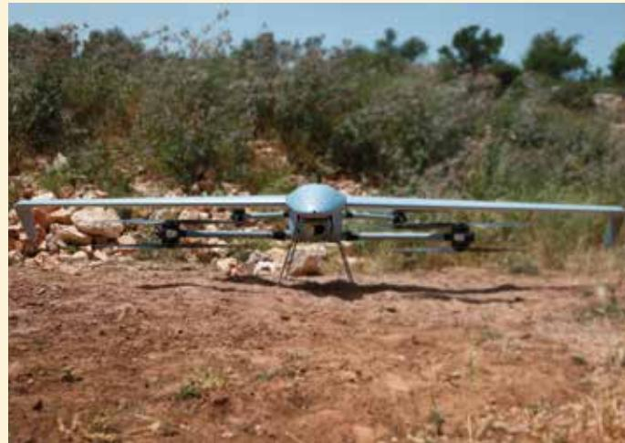
Taking an airframe with a classic wing and adding to it some rotors that can transform it into a rotorcraft for limited periods of time, allowing for persistent surveillance into areas where loitering UAVs cannot provide it, as well as multiple landing and take-offs in the operational area, and you get what Aeronautics of Israel defines a UHP, for Unmanned Hovering Plane.
